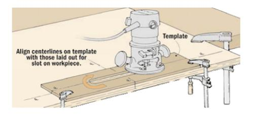
After cutting the template to size, you're ready to lay out the slot. The idea is to centre the slot on the width and length of the template, leaving the centrelines visible. (Later, they'll serve as reference lines so you can align the template on the work piece easily.) Now creating the slot is just a matter of drilling two end holes and roughing out the waste with a jig saw. Then sand (or file) up to the layout lines to provide a smooth edge for the bearing to ride on.
