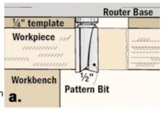
Before using the template, you'll need to lay out the centrelines for the slot on the work piece. Just be sure these lines extend far enough so they won't be covered once the template is positioned. Then rough out the slot in the work piece with the pattern bit and the router.
